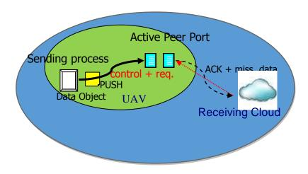
Figure 1: Operation with buffering at the Active Peer Port
