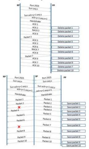
Figure 2: Sequence diagram of selected repeat protocol
