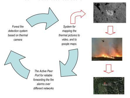
Figure 3: System Architecture on the UAV (left) and mapping of the thermal pictures to the video pictures, and to Google maps on the CMC cloud (right).
