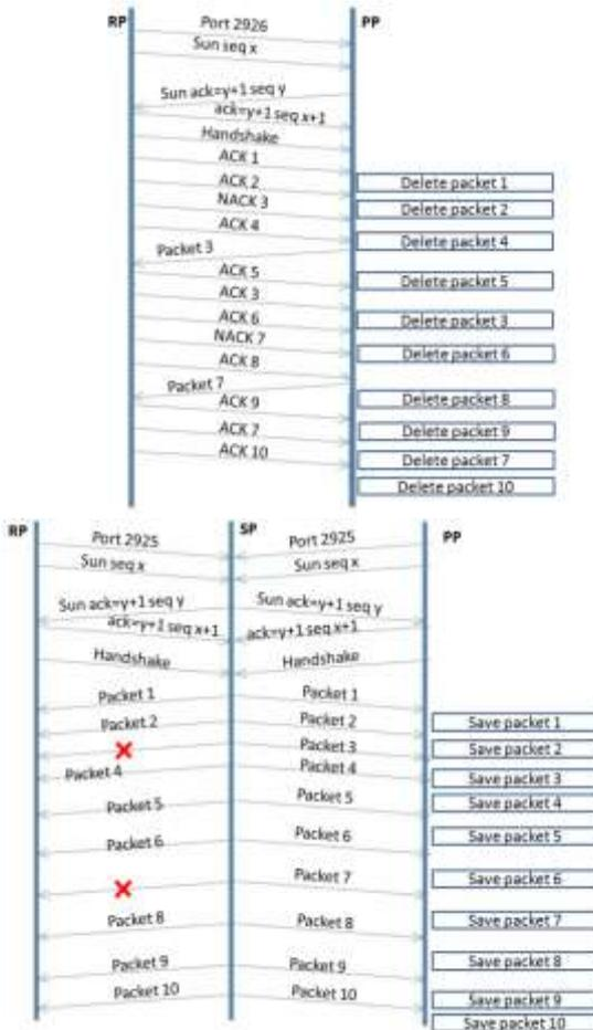
Figure 2: Sequence diagram of selected repeat protocol
