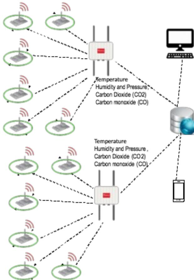
**Figure 7** Basic structure of wireless sensor network
