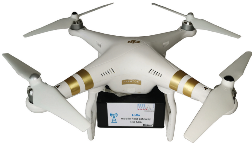
ASPIres mobile field gateway on a drone
