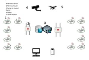
**Figure 1** Design of advanced system for monitoring of forest area and early detection of forest fires using drones, camera, and wireless sensor network
