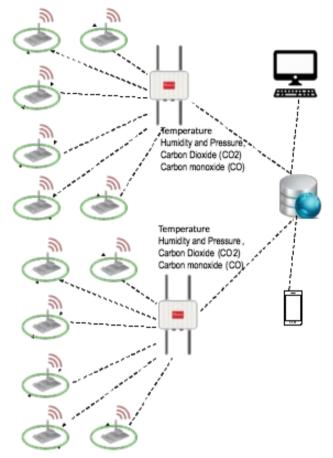
Figure 7 Basic structure of wireless sensor network
